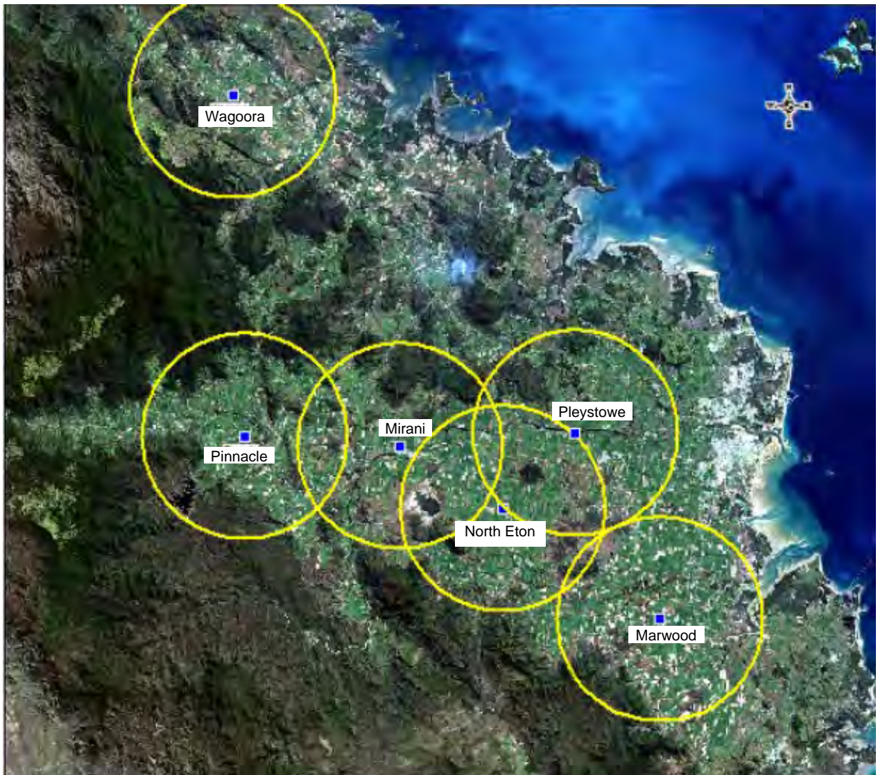
Figure 28 Mackay Sugar GPS base station network coverage map (2008)
