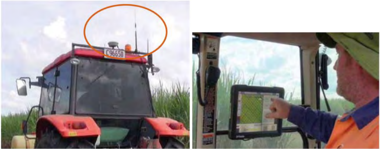
Figure 27 Differential GPS receiver mounted on tractor and in-cab GPS guidance display
